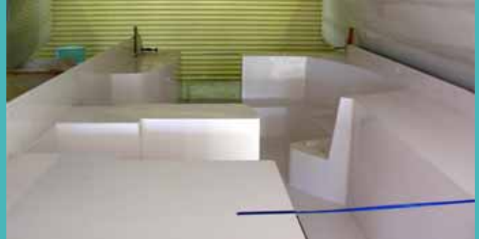
The saloon is one moulding that drops in or can be cut
