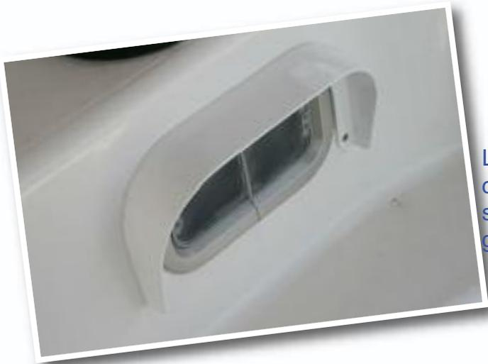
Leaving one of the aft facing Portlights open can find you with a wet bed. Greg made this simple looking visor which fits snugly, looks good and best of all keeps the elements out.
