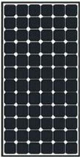
Utilizing 72 next generation SunPower all-back contact solar cells and an optimized panel design, the SunPower 215 delivers an unprecedented total panel conversion efficiency of 17.3%. The 215 panel's reduced voltage-temperature coefficient and exceptional low-light performance attributes provide far higher energy delivery per peak power than conventional panels.
