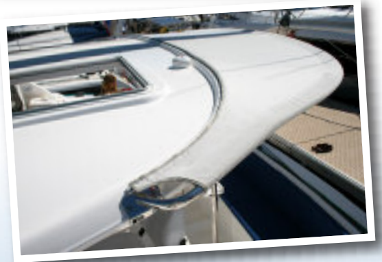
Right: A nice clean method of extending the saloon roof if required
